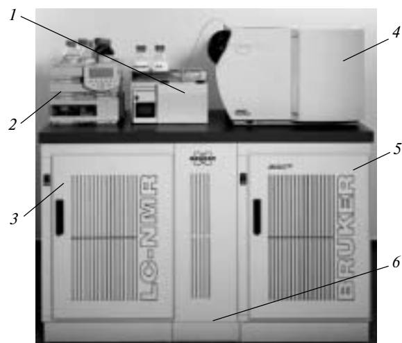
Fig. 1. LC—NMR—MS spectrometer combination. 1, B-NMI Bruker NMR—MS interface; 2, HP1100+ autosampler; 3, LC—NMR interface, UV DAD; 4, Esquire 3000 mass spectrometer; 5, Avance 500 NMR spectrometer; 6, vacuum pump of the mass spectrometer.
